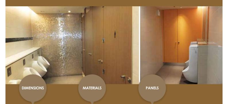
Cubicles' 2000mm overall height design includes a 150mm floor clearance. Its width and depth are tailored to meet your preferences and to adapt to individual site conditions. Standard design combines the use of solid compact laminate panel (phenolic core), natural anodized channel, and stainless steel accessories. Other options are available.
